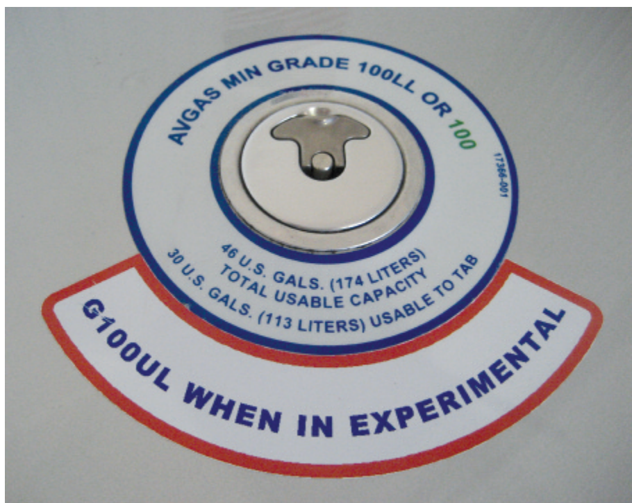
This unique label on the experimental aircraft's wing calls attention to GAMI's special G100UL fuel.
