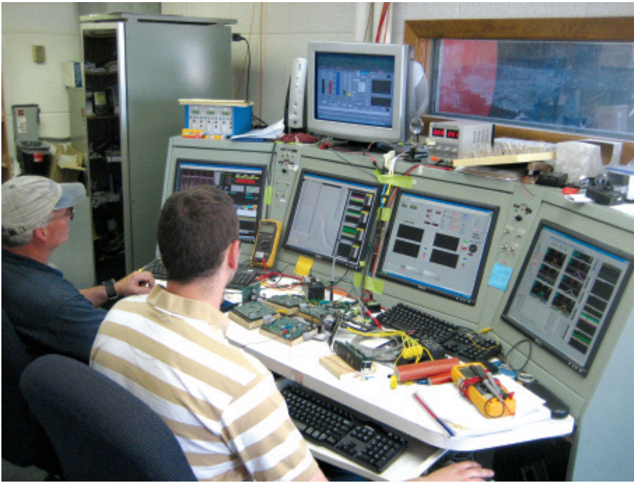
Engineers man the control console, which features computers, monitors, and instruments that process and display every aspect of the engine's performance during testing.
